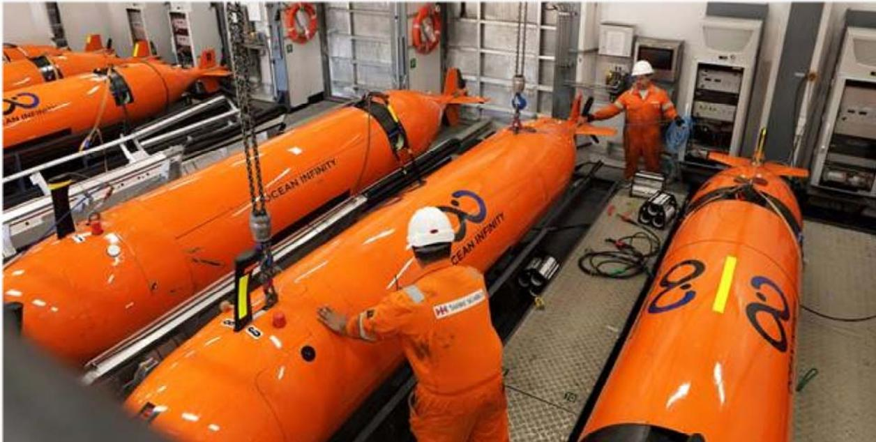
*Ocean Infinity's AUVs being prepared to autonomously map the ocean floor, aboard Seabed Constructor*
